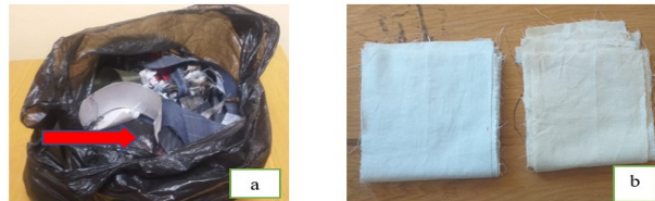
Figure 1: Gabardine waste and Cotton fabric materials used in the experiments. a. shows the gabardine waste and b. shows the cotton fabric material.
